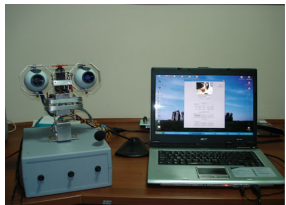
Fig. 3 Robotic head—WHA8030 of Dr. Robot [1]
